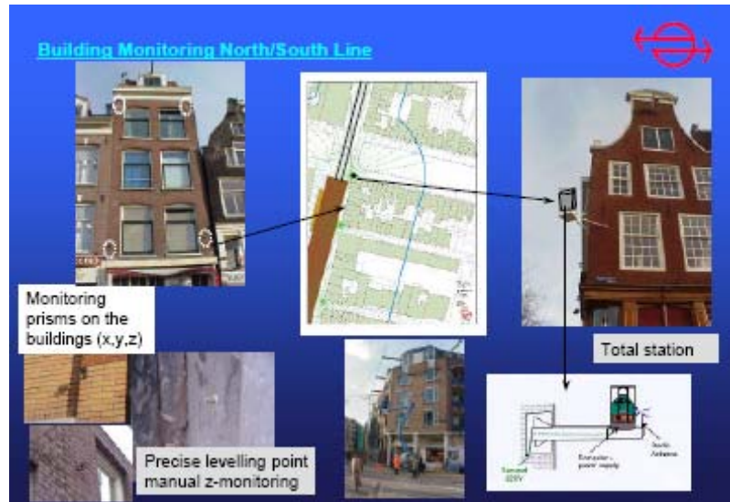
Figure 7: Monitoring system North/South metro line.
